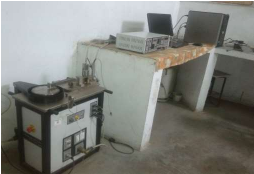
Fig. 1 PIN ON DISK (TR-20LE-PHM-400) (Industrial Engineering lab, GNDEC, Ludhiana.)
