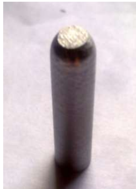
Fig. 2 Pin specimen made of H11 steel (before wear) Fig 3 Pin specimen made of H11 steel (after wear)
