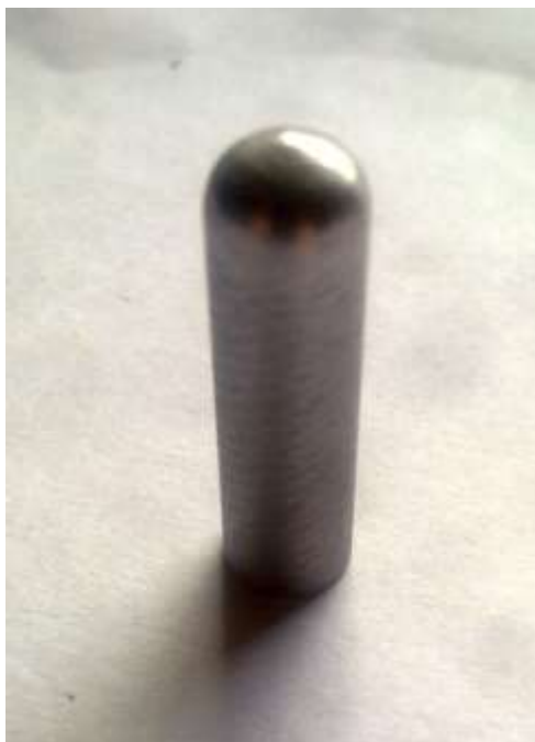
Fig. 2 Pin specimen made of H11 steel (before wear) Fig 3 Pin specimen made of H11 steel (after wear)
